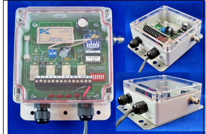
Dimensions (with mounting plate) 6.3" L x 4.8" W x 2.3" H (120VAC powered unit shown)
